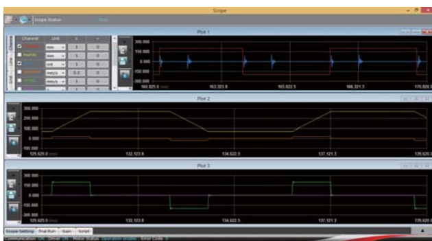
- Scope provides a real time monitor of driver information. - User could inspect motion detail without an oscilloscope.
